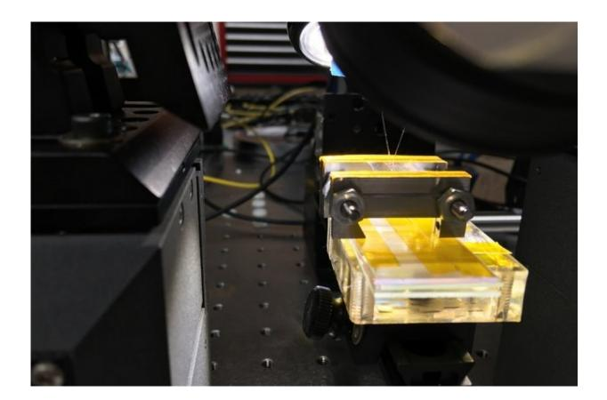
A view of the lab setup that was used to test the new materials, demonstrating that they could be stretched and flexed without losing the ability to confine light beams and carry out photonic processing. Credit: Massachusetts Institute of Technology
