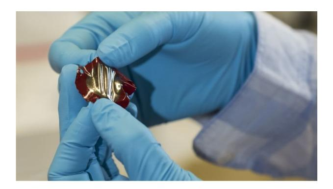
A sample of piezoelectric rubber. Credit: Swiss Federal Laboratories for Materials Science and Technology
