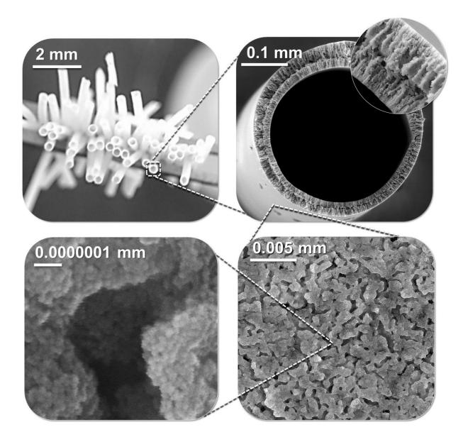
A tube-shaped bijel filter. Researchers at the University of Pennsylvania's School of Engineering and Applied Science have a new way of making polymer filters out of bijels, or bicontinuous interfacially jammed emulsion gels, that allow functional nanoparticles to adhere to the surface of the polymer. They tested their method with nanoparticles that prevent the build-up of biofilms. Credit: University of Pennsylvania
