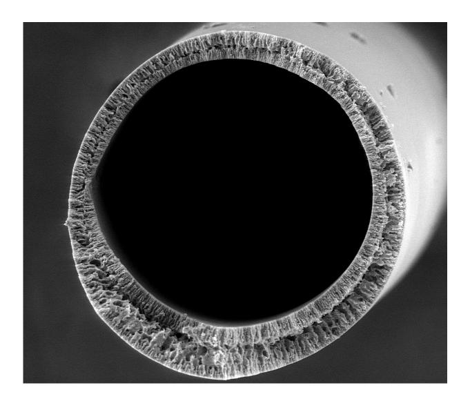
A tube-shaped bijel filter. Researchers at the University of Pennsylvania's School of Engineering and Applied Science have a new way of making polymer filters out of bijels, or bicontinuous interfacially jammed emulsion gels, that
