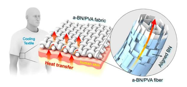
In the thermal regulation textile, the highly aligned nanofibers act as efficient heat transfer pathways. Credit: Gao et al. ©2017 American Chemical Society
