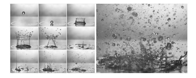
Impingement and vaporization of a 5-millimeter water droplet onto a 3-millimeter film of hot canola oil. The image to the right, shot just half a second after the water first contacts the oil, shows a plethora of droplets that are released. Some droplets are submicron and can remain airborne for more than 30 minutes. Credit: Marston Research Group, Texas Tech University
