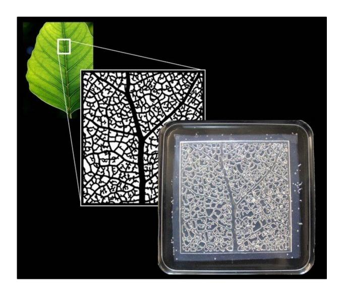
A vascularized polymer inspired by the vein structure of a leaf. The vascular channels within the polymer can be used to introduce different types of
