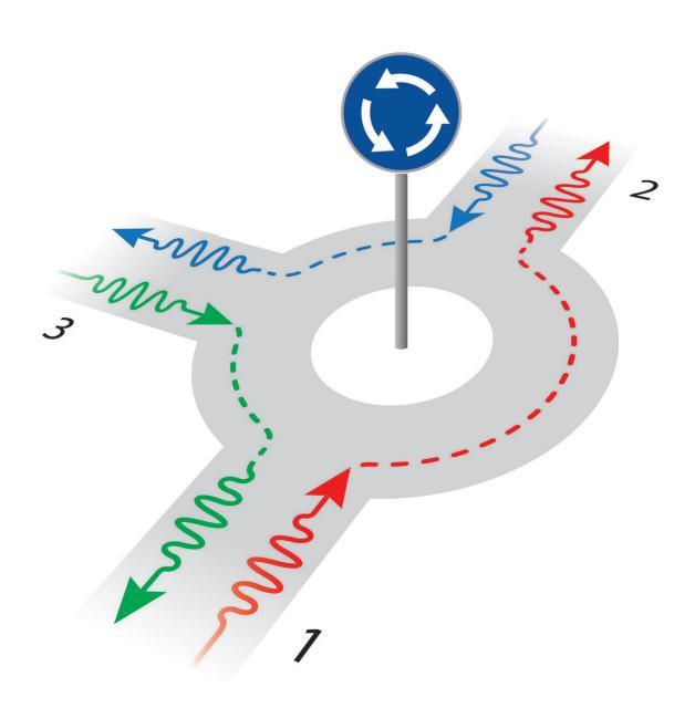
The new nonreciprocal device acts as a roundabout for photons. Here, arrows
