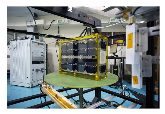
Technology CubeSat GomX-4B undergoing 'degaussing' – reducing the magnetic fields of its component parts by applying an opposite magnetic field to it – at ESA's Mobile Coil Facility at its technical centre in the Netherlands in June 2017. Such a magnetic cleaning procedure is needed to optimise the performance of the 'magnetotorquers' the nanosatellite will use for attitude control, with electromagnets reacting to Earth's magnetic field. Credit: European Space Agency
