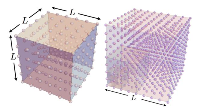
While quantum entanglement usually spreads through the atoms in an optical lattice via short-range interactions with the atoms' immediate neighbors (left), new theoretical research shows that taking advantage of long-range dipolar interactions among the atoms could enable it to spread more quickly (right), a potential advantage for quantum computing and sensing applications. Credit: Gorshkov and Hanacek/NIST
