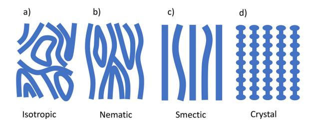
Cartoon of electronic liquid-crystal phases at half-filling. This research indicates a transition from nematic (b) to smectic (c) phases. Credit: Purdue University
