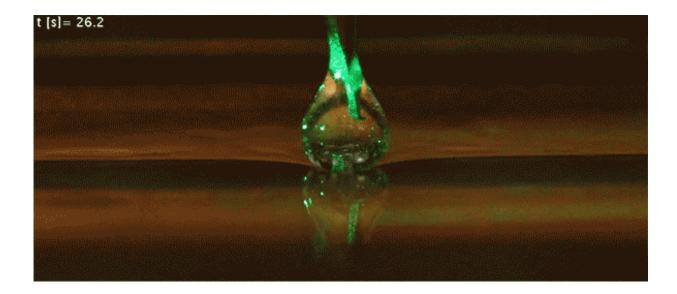
Visualization of recirculation vortices in the pending drop that is sitting on a warm bath. The temperature difference generates a recirculating flow that is visualized by shining a green laser light to the fluorescent particles that are added as passive tracers for sake of flow visualization. Credit: Massachusetts Institute of Technology
