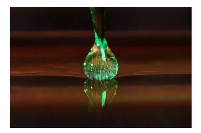
Visualization of vortices in a drop of silicone oil sitting on a warm bath. The temperature difference generates a recirculating flow that is visualized by shining a green laser light on fluorescent particles that are added as passive tracers within the drop. Credit: Massachusetts Institute of Technology
