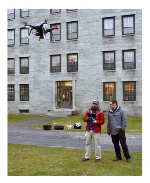
In this Nov. 14, 2017 photo, Dartmouth's Chad Hill, left, and Jesse Casana watch as their drone equipped with a thermal imaging camera flies around the site of a Shaker Village in Enfield, N.H. The camera uses the heat differences between stone and the soil surrounding it to identify structures below the surface, which then can be further explored. The two researchers are using the equipment at six archaeological sites around the world. (AP Photo/Michael Casey)
