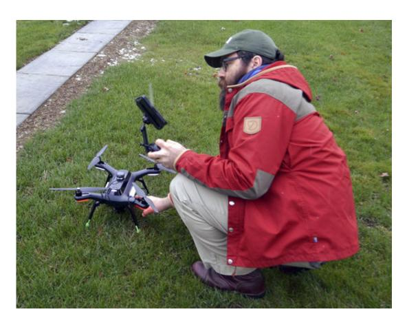
In this Nov. 14, 2017 photo, Dartmouth's Chad Hill studies a screen showing data collected by a drone at a the site of a Shaker Village in Enfield, N.H. Hill and Jesse Casana are using drones equipped with thermal imaging cameras to study a half-dozen archaeological sites around the world. The cameras use the heat differences between stone and the soil surrounding it to identify structures below the surface, which then can be further explored. (AP Photo/Michael Casey)
