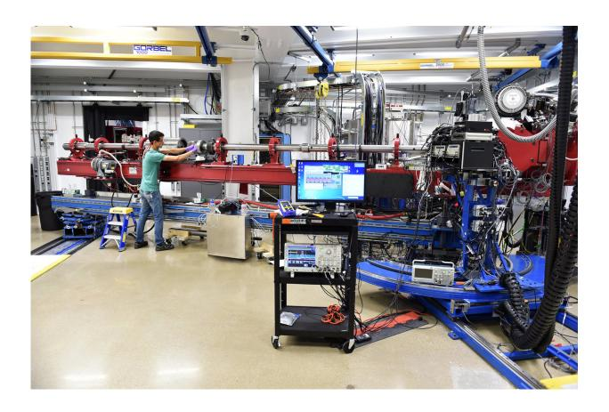
The DCS two-stage gas gun used for experiments is linked to the APS x-ray beam. Credit: Washington State University
