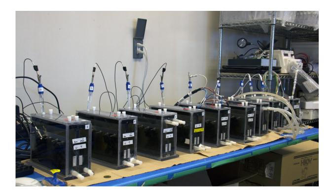
MFCs in the OIST Biological Systems Unit lab containing treated and untreated wastewater from the Okinawa Prefecture Livestock and Grassland Research Center. Credit: OIST
