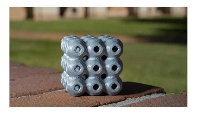
A schwarzite created on a 3-D printer by materials scientists at Rice University makes real a mathematical theory formed more than 100 years ago. The curved surface repeats throughout the structure, which showed excellent strength and deformation characteristics in tests at Rice. Credit: Jeff Fitlow/Rice University
