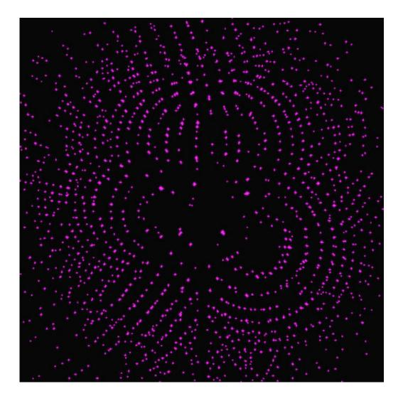
Diffraction image of a protein crystal in polychromatic, 'pink' X-rays. Compared to monochromatic X-ray diffraction images, the polychromatic image contains much more information and fewer crystals are required to determine the protein's structure. Credit: DESY, Max Wiedorn
