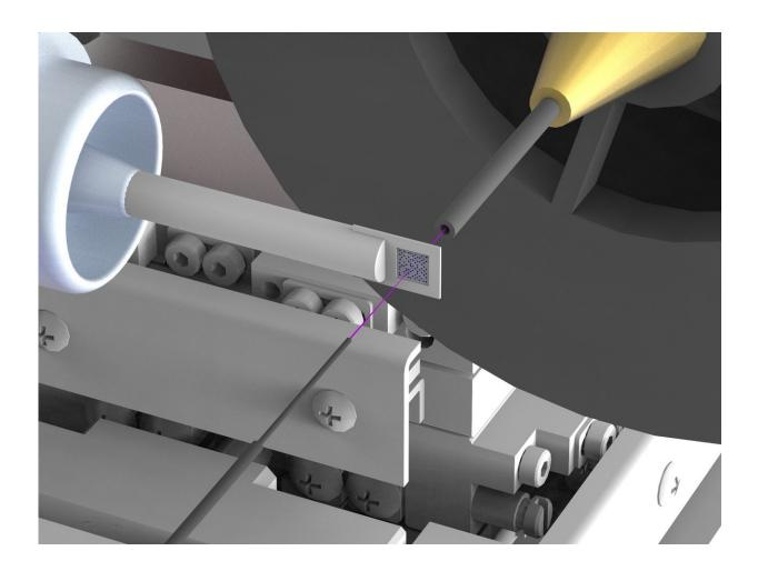
A newly developed set-up tremendously reduces background scattering in X-ray structure analysis of biomolecules like proteins at synchrotron X-ray sources. Scattering often hampers high resolution structure determinations. To achieve this, the X-ray beam (highlighted in pink) is enclosed in thin metal capillaries shortly before and behind the sample and the air immediately surrounding the sample is replaced by a stream of helium gas. Credit: DESY, Julian Bergtholdt
