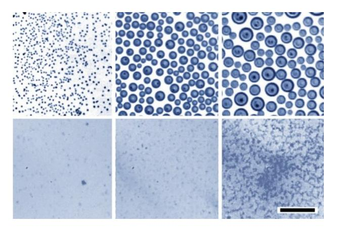
Optical images demonstrate that when water droplets condense on an oil bath, the droplets rapidly coalesce to become larger and larger (top row of images, at 10-minute intervals). Under identical conditions but with a soap-like surfactant added (bottom row), the tiny droplets are much more stable and remain small. Credit: Massachusetts Institute of Technology
