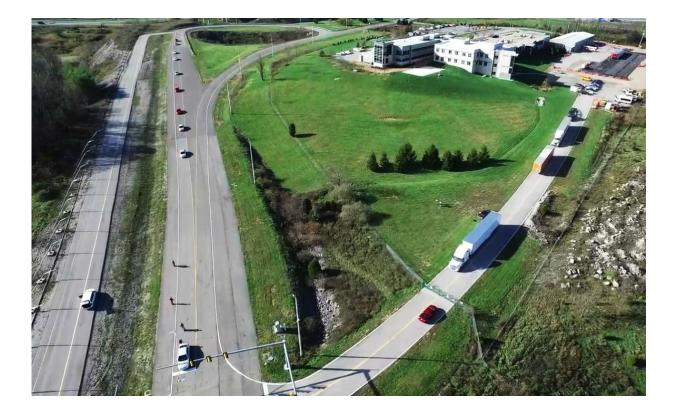
In video footage captured by a drone helicopter, volunteer drivers (left) approach a traffic light on the Virginia Tech Transportation Institute Smart Road as part of an experiment on optimal car spacing. Researchers in the Department of Biomedical Engineering and Mechanics discovered that packing tightly at traffic lights does not increase a driver's chances of being able to pass through the light before it turns red again. Credit: Virginia Tech
