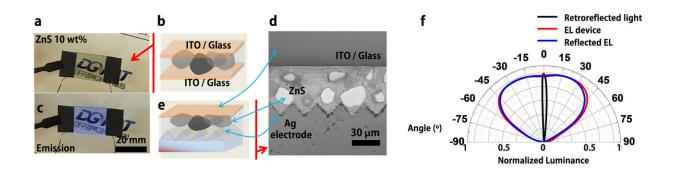
Structure and characteristics of electroluminescent device using recursive reflection structure. Structures (a~e) and viewing angle characteristics (f) of an electroluminescent device using a retroreflective structure. It exhibits a wide light reflection characteristic (Reflected EL) of -60  $^{\circ}$  and 60  $^{\circ}$  when viewing angle characteristics are evaluate. Credit: Daegu Gyeongbuk Institute of Science and Technology (DGIST)
