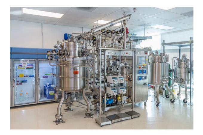
A bioreactor at Berkeley Lab's Advanced Biofuels and Bioproducts Process Demonstration Unit (ABPDU) was used to scale the growth of the mixture of bacteria to 300 liters. Credit: Roy Kaltschmidt/Berkeley Lab
