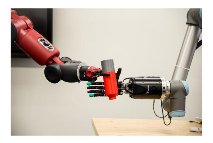
A first-of-its-kind bioengineered robotic hand will grow and adapt to its environment. This "living" robot will have its own peripheral nervous system directly linking robotic sensors and actuators. The research team is creating a living pathway from the robot's touch sensation to the user's brain to help amputees control the robotic hand. Credit: Florida Atlantic University
