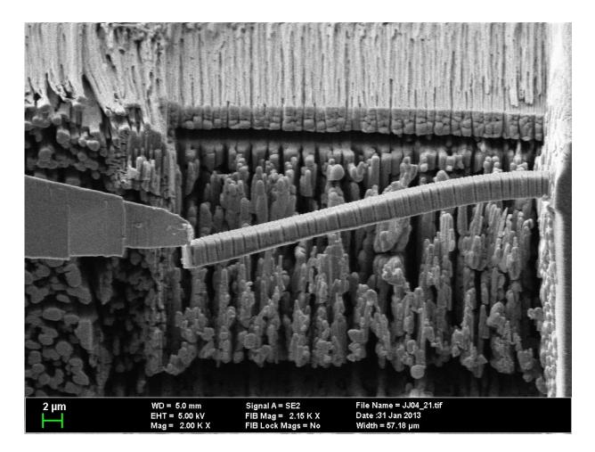
Bending experiment on elastic cement in a scanning electron microscope, enlarged 2,000 times Bar-shaped micro-structure precision-cut from nanostructured cement using an ion beam, bends under the pressure of a micromanipulator without breaking (micro-manipulator left in the picture). Credit: Dr Zhaklina Burkhard
