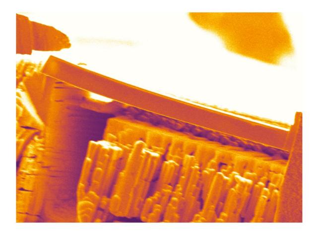
Micro-manipulator bending a cement microbar. Credit: University of Konstanz
