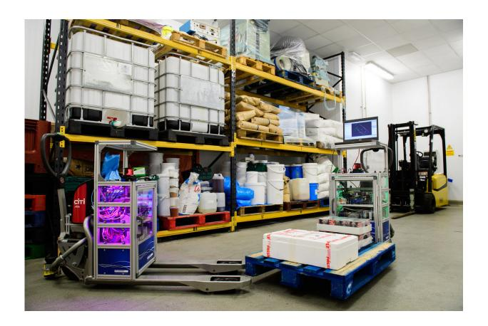
The autonomous forklift trucks are designed to operate in is to enable deployment of next generation automated guided vehicles (AGVs) into current warehouse facilities to support tasks such as packing, palletising and transporting goods. Credit: Chris Vaughan/ University of Lincoln
