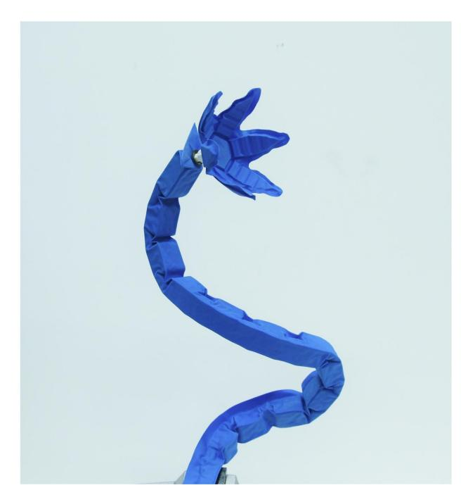
Snake-like robotic arm with a flower-like gripper driven by a single vacuum source. Credit: Shuguang Li
