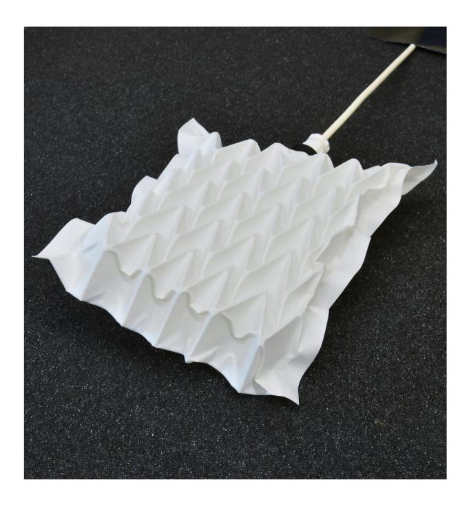
A vacuum-driven artificial muscle producing complex out-of-plane motion
