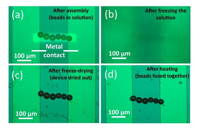
After using optoelectronic tweezers to assemble a line of solder beads (a), the researchers froze the liquid (b) and then reduced the pressure so that the frozen liquid turned directly from a solid into a gas, drying out the device (c). They then heated the beads to fuse them into an electrical connection. Credit: Shuailong Zhang
