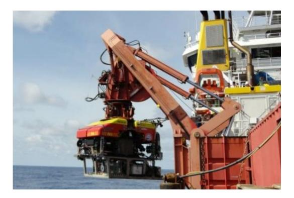
The remotely operated vehicle, deployed from the James Cook research vessel, used to recover environmental samples from previously unexplored regions of the Atlantic Ocean sea bed. Credit: University of Bristol
