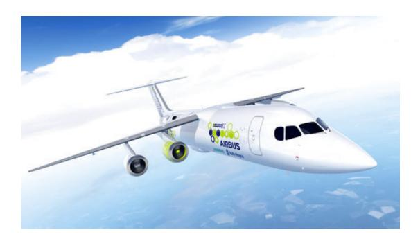
The artist rendering provided by Airbus on Tuesday, Nov. 28, 2017 shows an Airbus e-FanX hybrid test plane. The aircraft will be flying with one electric turbofan motor and 3 conventional engines. The electric power for the electric engine is being produced by a turbine within the plane that serves as a generator. (Airbus via AP)
