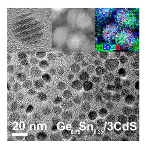
High-resolution and elemental mapping electron micrographs of near-infrared active GeSn/CdS nanocrystals. Credit: Ames Laboratory
