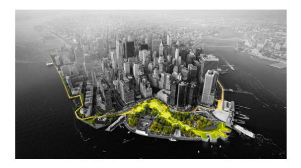
This illustration provided by Rebuild by Design in October 2017 shows a flood-mitigation design for the Manhattan borough of New York. The BIG U proposal calls for a 10-mile protective system around the low-lying southern part of the island. The proposal is part of the Rebuild by Design competition to create infrastructure that would protect coastal areas affected by Superstorm Sandy. (The BIG Team/Rebuild by Design via AP)
