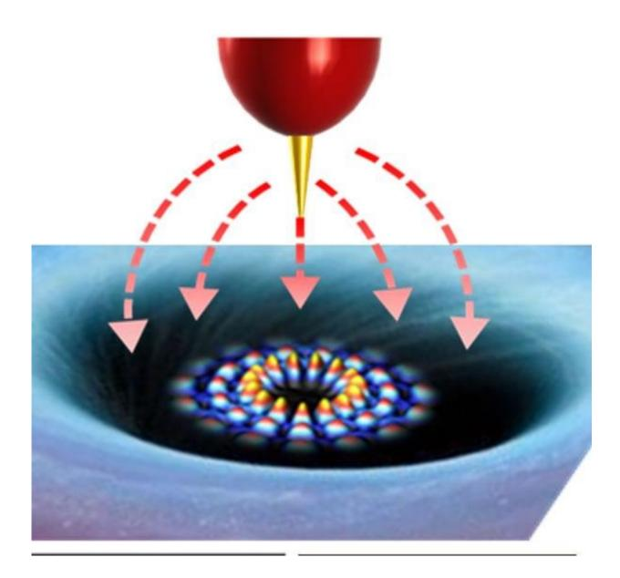
A sharp tip creates a force field that can trap electrons in graphene or modify their trajectories, similar to the effect a lens has on light rays. Credit: Yuhang Jiang/Rutgers University-New Brunswick
