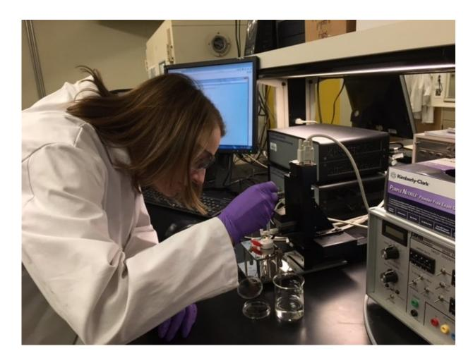
Postdoctoral associate Melanie Rudolph pours electrolyte onto a thin-film polymer for experiments on electron transfer reactions. Credit: University of Arizona
