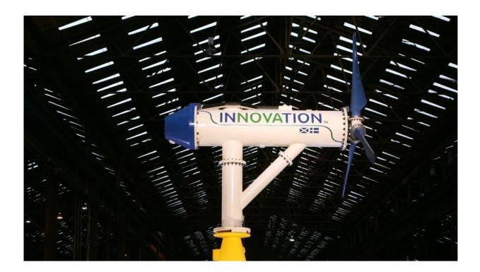
The sea's movements can be utilised to create electricity through underwater turbines. Credit: Nova Innovation/ EnFAIT
