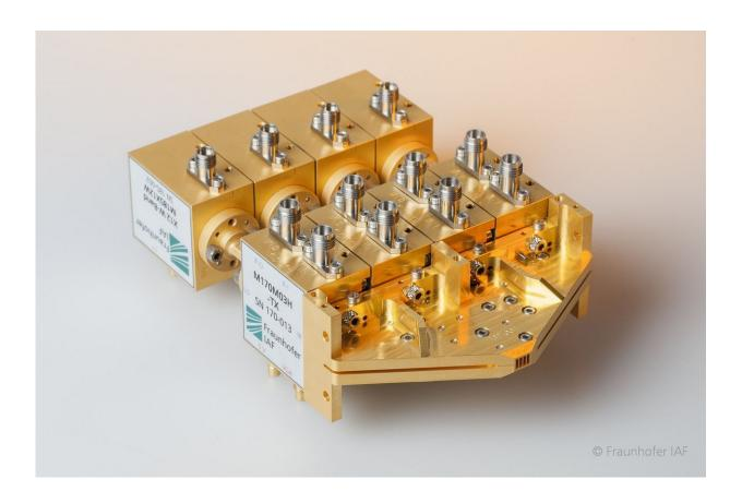
Functional prototype of a 300 GHz multichannel wireless system. Credit: Fraunhofer-Gesellschaft
