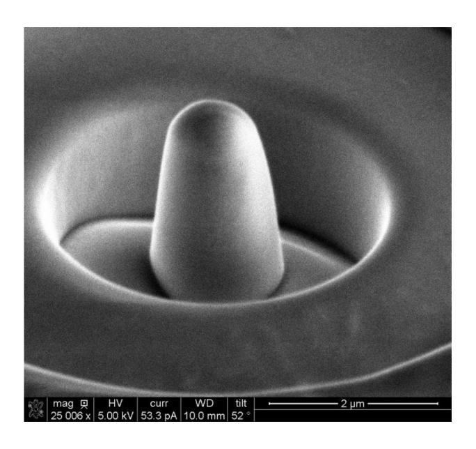
A representative cement micropillar sample imaged by scanning electron microscope. Samples like this one are key to the use of a 'micropillar
