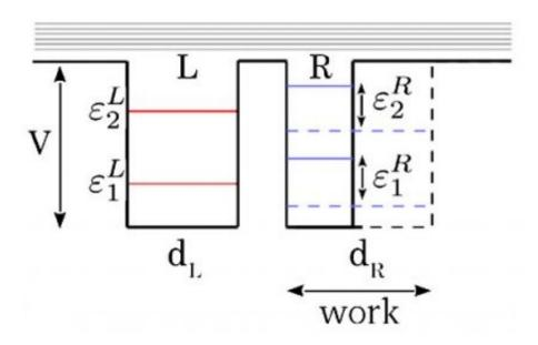
In this double quantum well system, the left well remains static while the right one oscillates, allowing work to be performed on the system. Credit: Sachtleben et al. ©2017 American Physical Society
