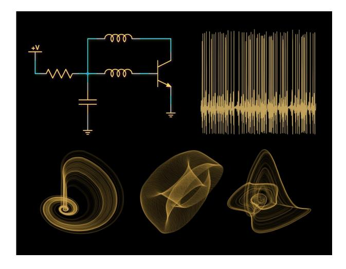
Chaotic voltage changes are common even for electronic circuits made up of only several elements. In the top left corner is a diagram of the simplest chaotic oscillator found by physicists from IFJ PAN in Cracow. On the right, a series of pulses showing a great resemblance to neural activity, generated by one of the newly discovered circuits. In the lower row several so-called attractors, illustrating the complexity of behaviour of the new circuits. Credit: IFJ PAN
