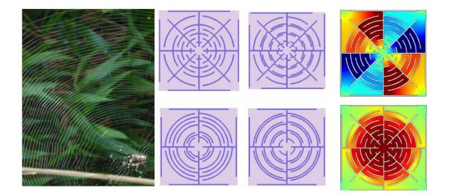
(Left) Photo of a natural spider web (by D. Krushinsky), along with illustrations of spider web-structured acoustic metamaterials (center), and figures of their acoustic dispersion and transmission spectra (right). Credit: Krushynska et al. ©2017 IOP Publishing
