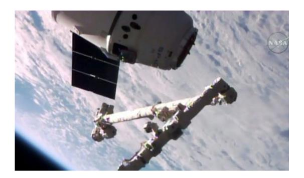
The Canadarm2 robotic arm is poised to grab the unmanned SpaceX Dragon cargo capsule in this NASA TV video grab from June 5, 2017
