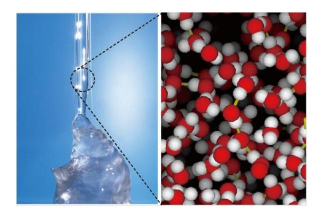
Figure 1. (Left) Supercooled water is frozen with shocks (Copyright: Takeshi Fujino, KOWA Corporation, Niigata, Japan) (Right) Snapshot of supercooled water calculated from our computer simulations (red: oxygen, white: hydrogen, yellow bond: hydrogen-bond). Credit: Osaka University
