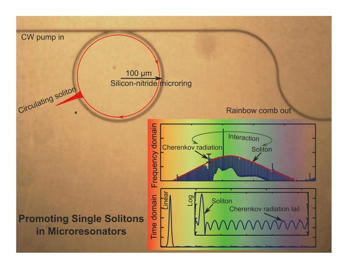
Purdue researchers have used tiny microrings (top left) to generate single pulses of light called solitons, an advance that could aid efforts to develop advanced optical technologies. Two graphs show the relationship between a phenomenon called Cherenkov radiation and production of single solitons. Credit: Purdue University photo/Chengying Bao
