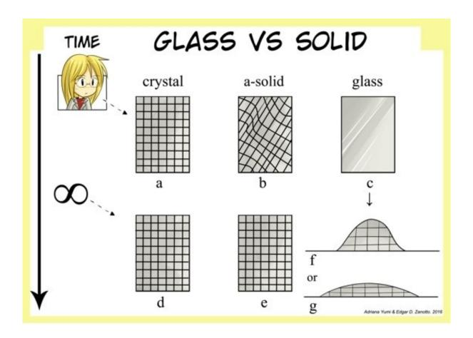
A crystal (solid), an amorphous solid and a glass on human time scale and their ultimate fates on an infinite time scale. Credit: FAPESP
