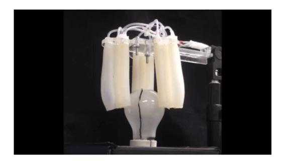
The soft robotic gripper is capable of screwing a light bulb in. Credit: University of California San Diego
