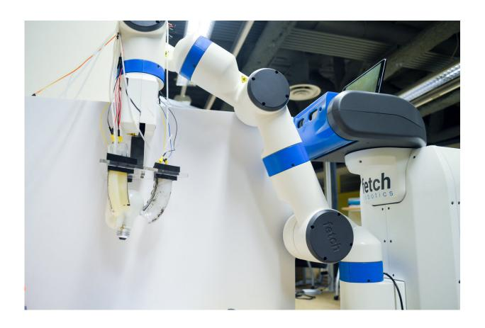
Researchers installed the soft robotic gripper on a Fetch Robotics robot in their lab. Credit: University of California San Diego
