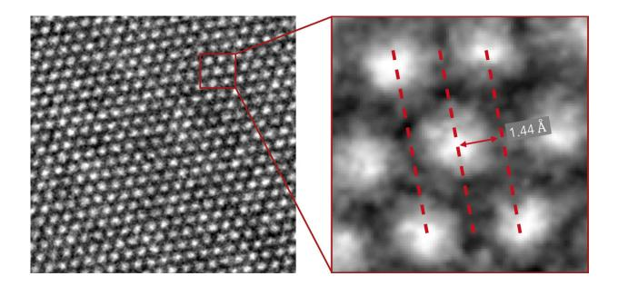
With cryo-EM, scientists were able to look at the way electrons bounced off the atoms in the dendrite, revealing the locations of individual atoms (left). They were even able to measure the distance between atoms (right). The spacing between these atoms shows that they are lithium. Credit: Y. Li et al., Science
