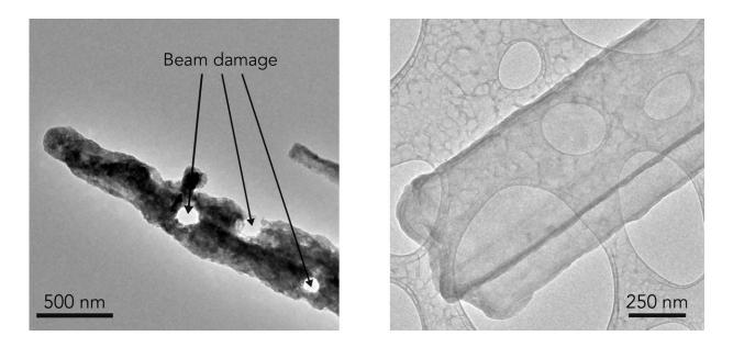
Left: In this room-temperature TEM image, exposure to air has corroded a lithium metal dendrite and the electron beam has melted holes in it. Right: In contrast, a cryo-EM image of a dendrite shows that freezing has preserved its original state, revealing that it's a crystalline nanowire with well-defined facets. Credit: Y. Li et al., Science
