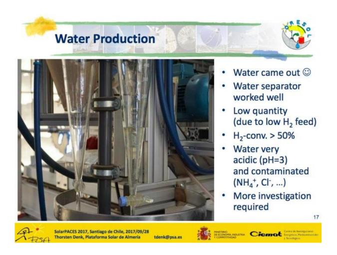
With the successful test of this solar reactor design, Denk has achieved the first step, creating H2O on the Moon using solar thermal energy. For the second step, solar electrolysis would break the H2O into hydrogen and oxygen. Credit: Thorsten Denk: Presentation at the International Annual SolarPACES Conference 2017
