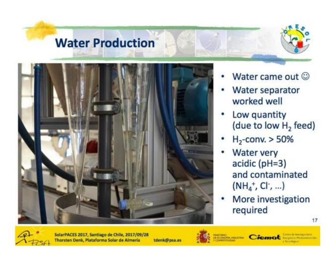
With the successful test of this solar reactor design, Denk has achieved the first step, creating H2O on the Moon using solar thermal energy. For the second step, solar electrolysis would break the H2O into hydrogen and oxygen. Credit: Thorsten Denk: Presentation at the International Annual SolarPACES Conference 2017
