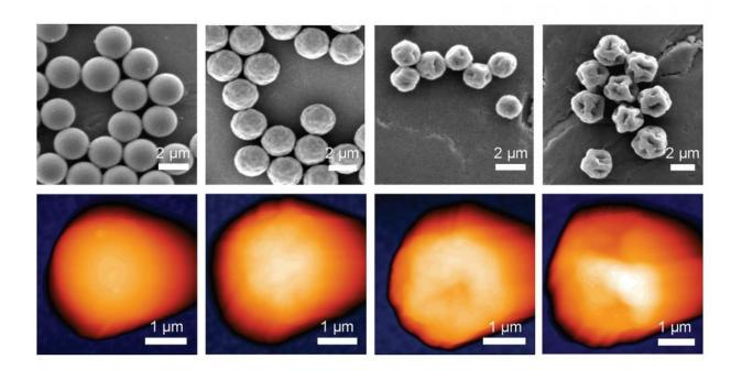
The top panel is a series of scanning electron micrographs for particles ranging from smooth to rough. The bottom panel is a series of atomic force micrographs showing the 3D topography of these particles, again ranging from smooth to rough, to demonstrate the extensive characterization of their surfaces. Credit: North Carolina State University
