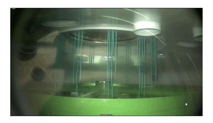
The first full-scale model of the P120C rocket motor that will propel Ariane 6 and Vega-C into orbit was cast and filled with inert propellant for intensive testing in Europe's Spaceport in French Guiana in September 2017. It is the largest single casting of a solid propellant motor ever achieved. The photo was taken by a camera inside the casing. Credit: ESA
