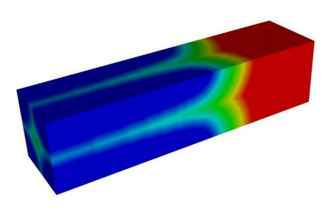
An illustration shows the growth of a lithium-deficient phase (blue) at the expense of a Lithium-rich phase (red) in a lithium iron phosphate microrod. Rice University researchers led a study that found defects in a common cathode material for lithium-ion batteries can potentially improve performance over perfect electrodes by allowing for lithium transport over much more surface area than previously thought possible. Credit: Mesoscale Materials Modeling Group/Rice University
