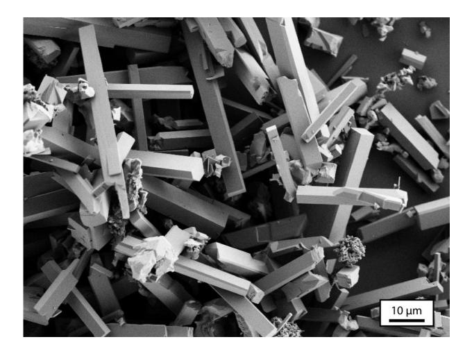
An electron microscope image shows microrod particles of the type used in a Rice University-led study of lithium transport in lithium-ion batteries. Credit: Linsen Li and Song Jin/University of Wisconsin Madison
