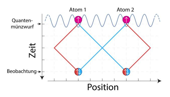
Two atoms, initially prepared in different locations, exchange their positions along the blue path, whereas no exchange occurs along the red path. In quantum mechanics, it is possible that the atoms take simultaneously both ways. As a result of such a tricky manipulation, it is fundamentally impossible at the end to determine the origin of the atoms, and their spin orientations (denoted by arrows) become entangled. Credit: Andrea Alberti/Uni Bonn
