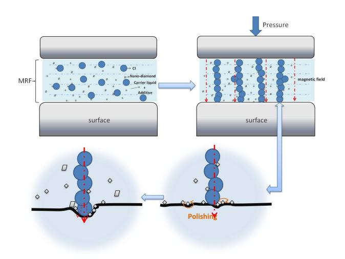
As the fragmented nano-diamond had a high hardness, the MRF on the surface of the ball during friction was not stable. Moreover, as the duration and the role of the load increased, pit and debris appeared on the ball surface. As the nanodiamond was lower-sized, additional nano-diamond and debris went into the pit and continued to further polish the surface, whereas the depth and diameter of
