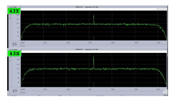
This animation shows the last 30 seconds of Cassini's X- and S-band radio signals as they disappeared from mission control on Sept. 15, 2017. The video has been sped up by a factor of two. Credit: NASA/JPL-Caltech
